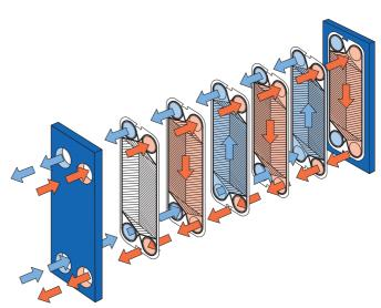
Flow principle of a plate heat exchanger
